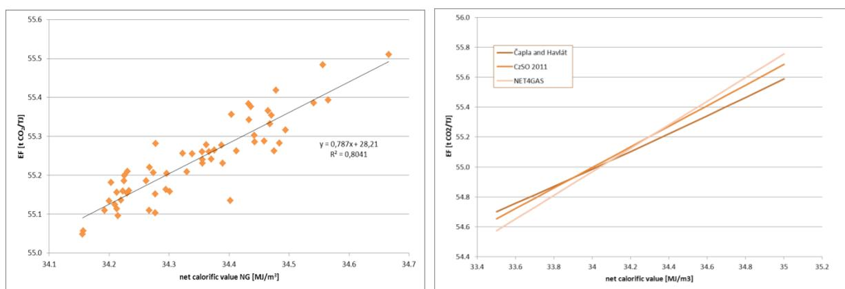
**Fig. A3 4 Correlation of EF [ $\text{t CO}_2/\text{TJ}$ ] and net calorific value of Natural Gas and Comparison of three approaches used for calculation**
