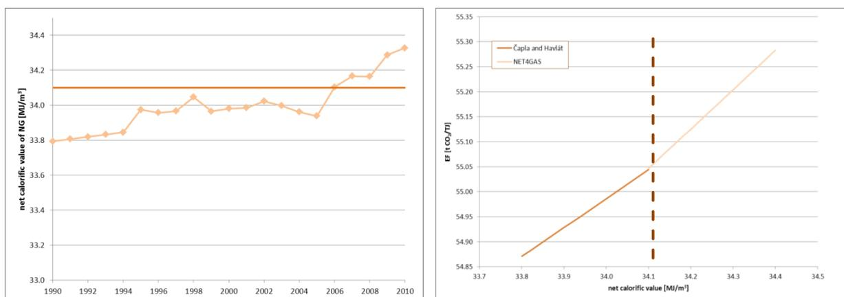
Fig. A3 5 Trend in Natural Gas NCV 1990 – 2010 and Correlation between NCV and EF combined from two approaches – Čapla and Havlát (NCV lower than 34.1 MJ/m<sup>3</sup>) and computed correlation on the basis of NET4GAS dataset (NCV higher than 34.1 MJ/m<sup>3</sup>)
