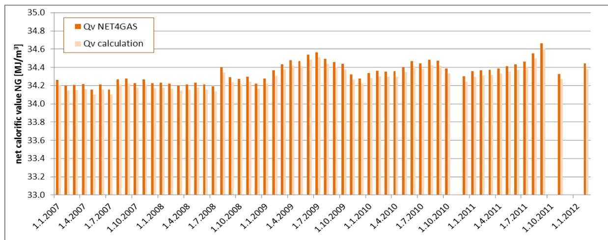
Fig. A3 3 Net calorific values given in NET4GAS Ltd. reports and net calorific values calculated on the basis of composition of Natural Gas in 1.1.2007 – 1.2.2012 (both values are given at 15°C)
